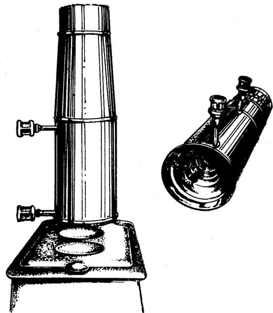
Fig. 1. Stovepipe water heater.
