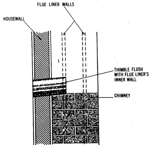
Fig. 18. Position of thimble with respect to wall of flue liner.
