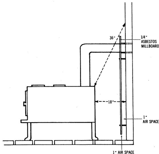
Fig. 2. Suggested minimum clearances from protected combustible walls.
