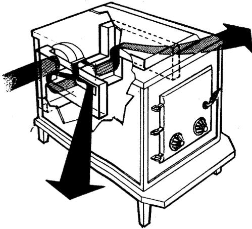
Fig. 7. Heat manifolds used in Nashua stove.
