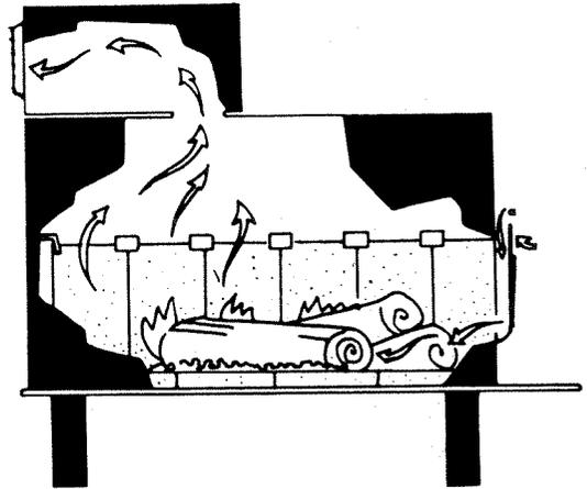
stove Co. (U.S. distributor and manufacturer), Bennington, VT 05201. The Canadian step stove (Fig. 61 and Table 6), unlike many others, has incorporated the principle of the horizontal baffle, just as in Scandinavian models. The steel plate is welded with "Deep-penetrating MIG welds, for completely airtight construction." The cast-iron door is sealed with gaskets, and is chambered for preheating intake air.
