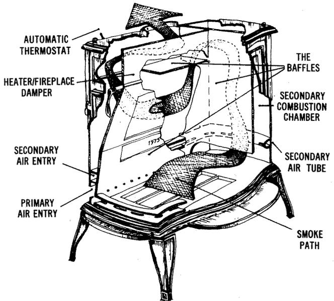
Fig. 12. Cutaway view of the Defiant stove.
