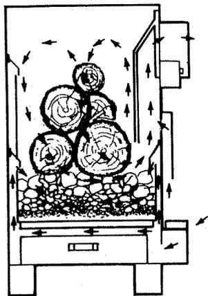
Fig. 11. Air-flow pattern in the Riteway 2000.
