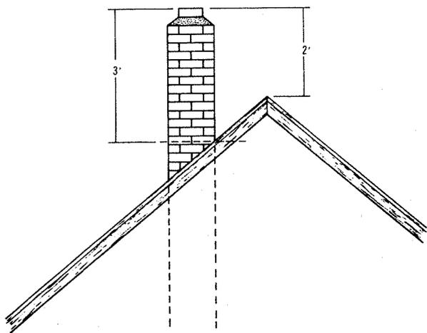
Fig. 3. Height of chimney above roof and ridge.
