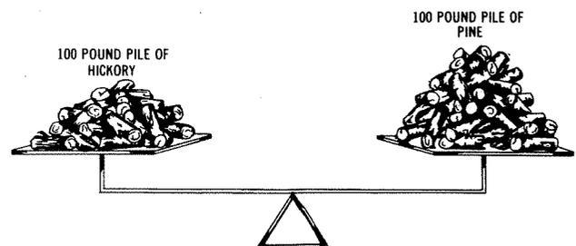
Fig. 2. One hundred pounds of hickory (left) balances an equal weight of pine (right), but takes up half the space.
