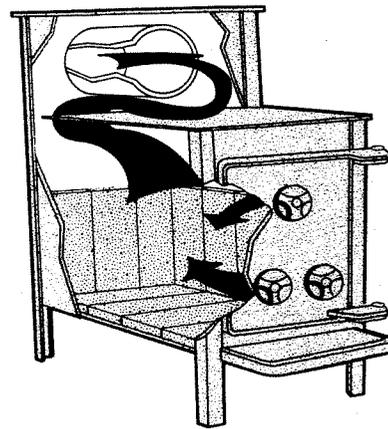
Fig. 14. Huntsman stove, showing recessed flue collar.
