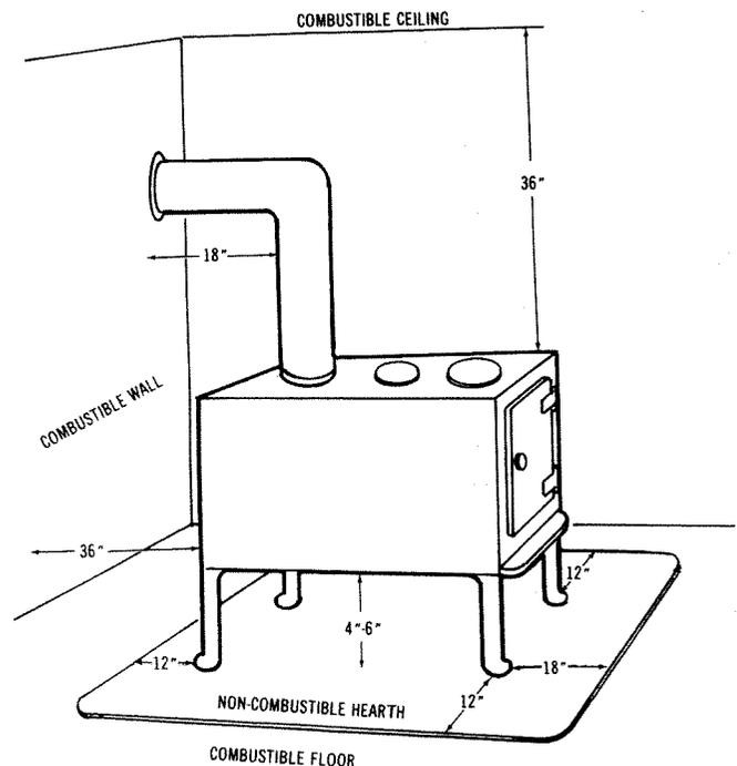
Fig. 1. Suggested minimum clearances from combustible surfaces.
