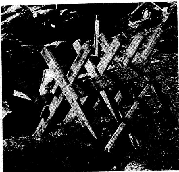
Fig. 5. Home-made, heavy-duty sawbuck.
