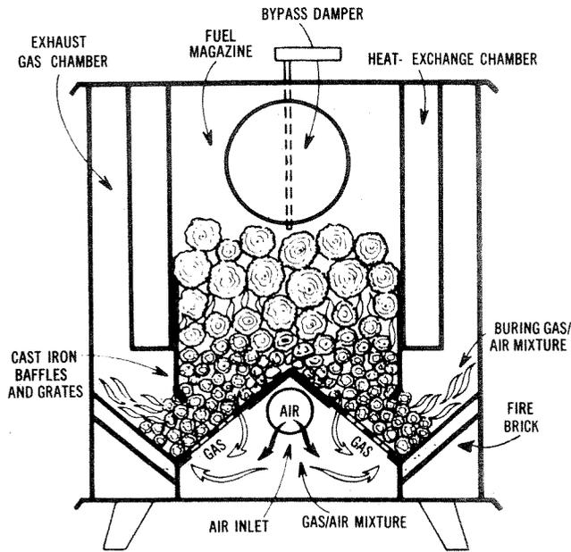
Fig. 15. Draft-flow pattern in Downdrafter box stove.
