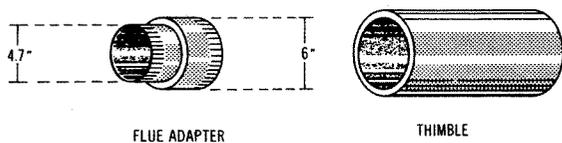
Fig. 2. Flue adapter (left) and thimble (right).
