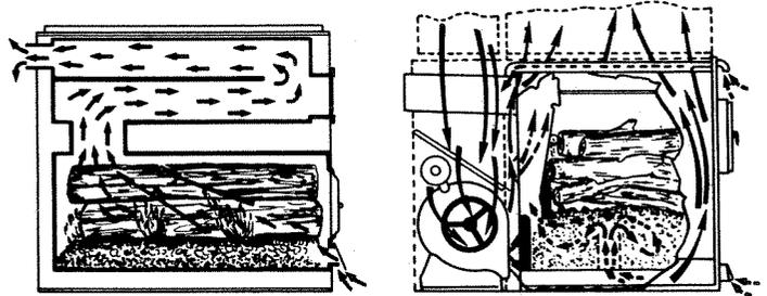
Fig. 80. Valley Comfort wood-burning furnace flow-patterns.
