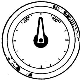
Fig. 6. Stack temperature should be 300-400 degrees F.
