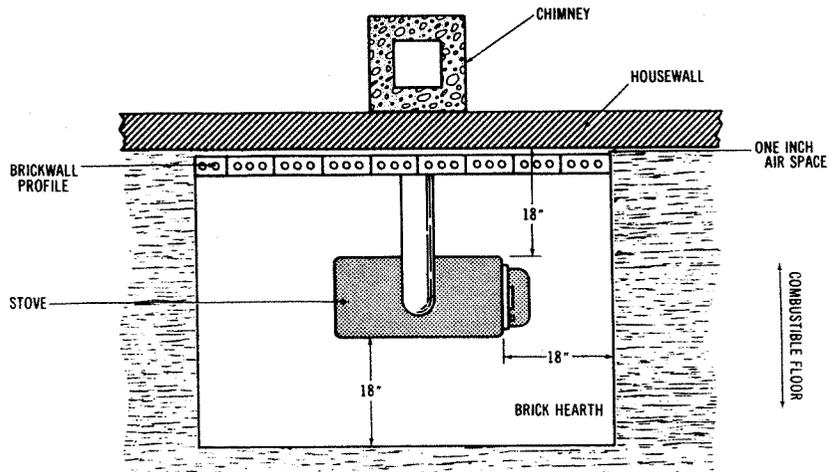
Fig. 10. Placement of stove on hearth area.
