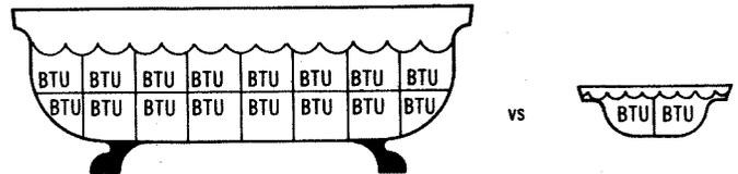
Fig. 1. There is more heat in a bathtub full of hot water than in a basin similarly filled.
