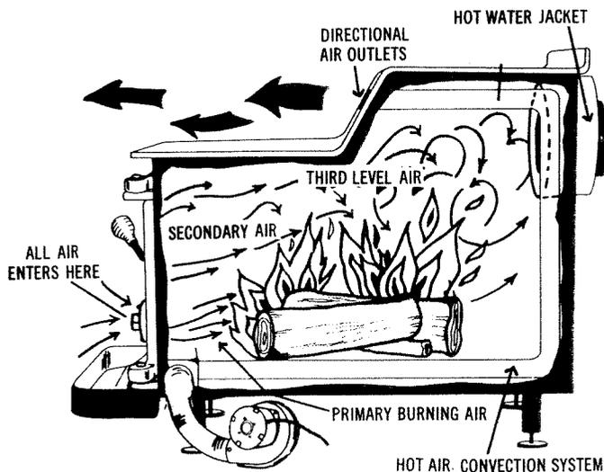
Fig. 13. Cutaway of All Nighter step stove.
